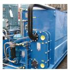
Screw pumps for the ship pump package:
