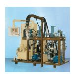
Pumps: L 20 with magnetic coupling. Pressure: approx. 170 psi.
