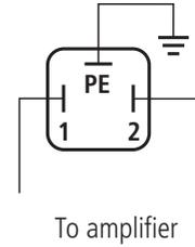
Plug-in connector to DIN EN 175301-803
