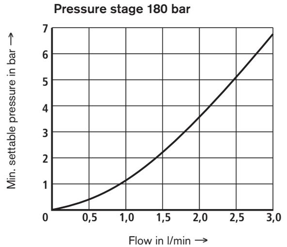
**Characteristic curves** (measured with HLP46,  $\vartheta_{oil} = 40 \text{ }^\circ\text{C} \pm 5 \text{ }^\circ\text{C}$  and **without** back pressure)
