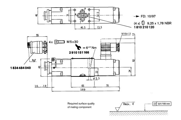
**Mounting hole configuration: NG6** (ISO 4401-03-02-0-94) For subplates, see catalog sheet RE 45053
