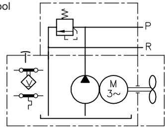
**Table 2 a:** Single circuit pumps with 3~phase motor
