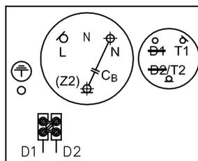
C<sub>B</sub> - Operating capacitor is not scope of delivery
