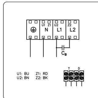
C<sub>B</sub> - Operating capacitor is not
