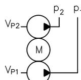
Both pumps work against different pressure simultaneously
