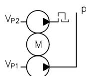
Only one pump works ( $V_{P1}$  against pressure,  $V_{P2}$  idles,  $p_1 = p$ )
