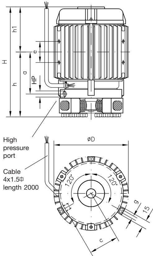
Single circuit pump (gear pump)
