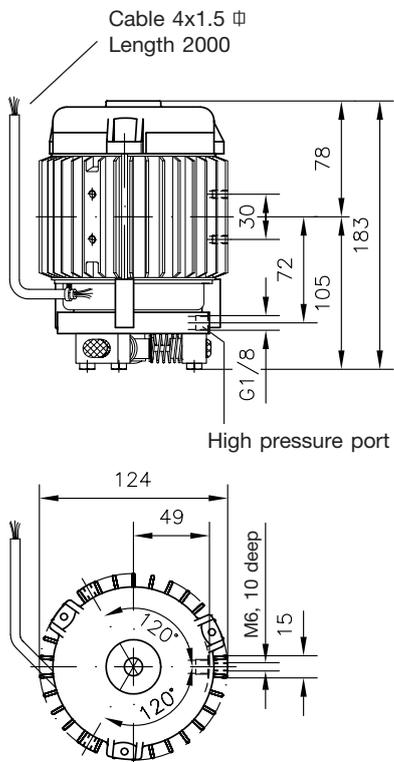
Single circuit pump (gear pump)
