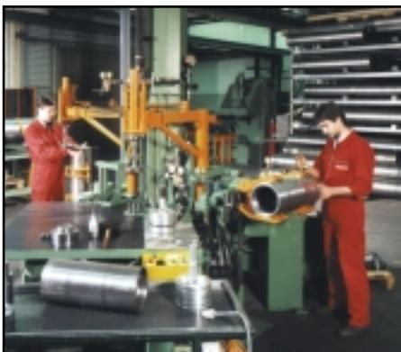
Assembly of piston accumulators
