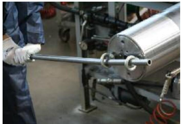
Gas pressure should always be discharged before the disassembly of an accumulator AP. Those accumulators have the oil and gas end caps threaded into the pipe. Always remove the gas cap first – identifiable by the gas valve or by a gas bottle connection.
