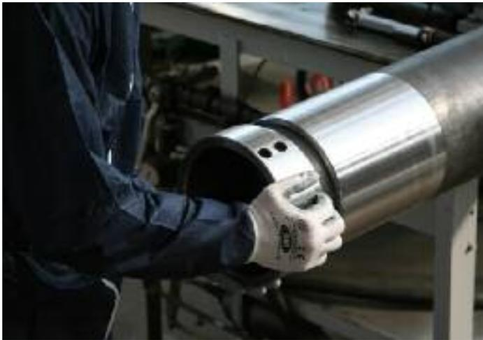
Coat all internal parts with clean hydraulic fluid before reassembly. In order to protect the piston seals and for ease assembly purposes, the use of a loading sleeve is recommended – details of a suitable loading sleeve can be provided by Epe. To minimize the risk of damage to the piston and seals, it is recommended that the replacement piston assembly should be installed with the accumulator pipe positioned vertically.
