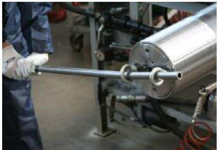
The O-ring and parbak ring, fitted to the accumulator end caps, have a flat face and a concave face to allow the ring and the parbak ring seaying correctly.
